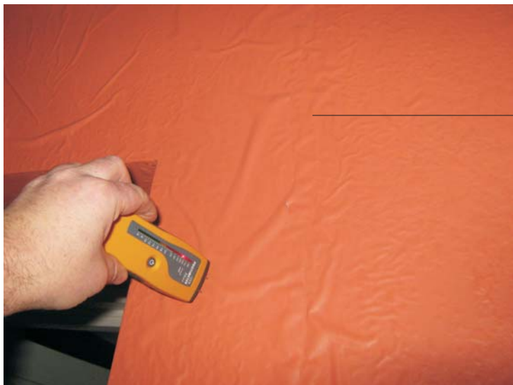
Photo 11 - saturated wall rear lobby - ground floor
